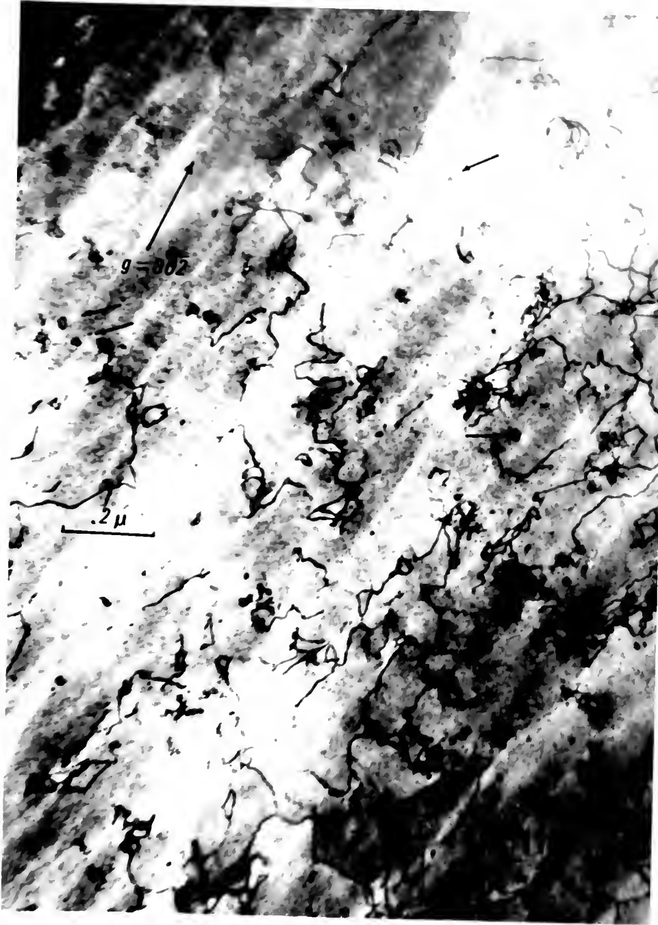
Figure 51.--Dark field electron micrograph of the same region with \vec{g} = (00\bar{2}) . Loops exhibiting a size change are arrowed.
